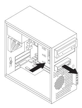
Figure 29. Removing the diskette drive
